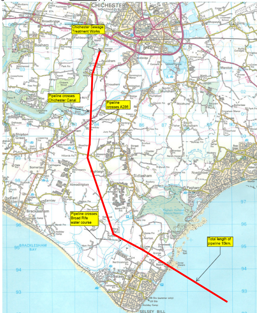
Figure 18 – OS map with indicative pipeline route from Chichester WwTW to the LSO
