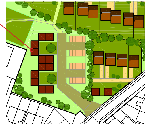
Extract of site plan for Thawcroft site, showing how work-live units could be integrated into a residential area.
