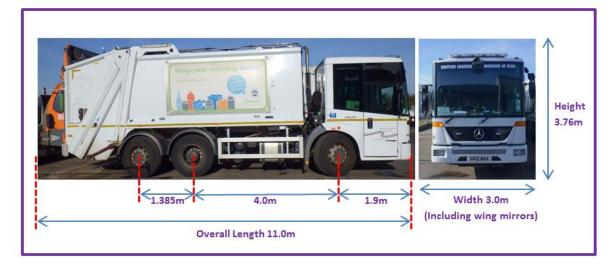
**3.** Fully laden collection vehicles weigh approximately 26 tonnes. Service manholes and road surfaces should be constructed with this in mind.
