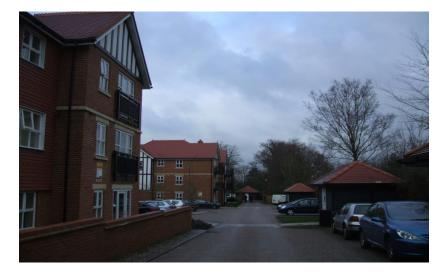
**Photo 2: Example of good practice - bin storage** A further example of good practice where the bin store is included in the main building but is at ground level. The store is close to the road so is accessible to the collection crew at all times and is not affected by parked vehicles. The refuse freighter can access the bin store without the need to reverse into the development.
