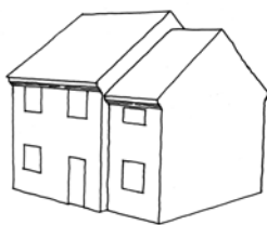
Side extensions should normally create a visual break between old and new,
