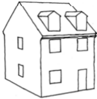
Dormer windows should be placed symmetrically and kept subordinate to the main roof
