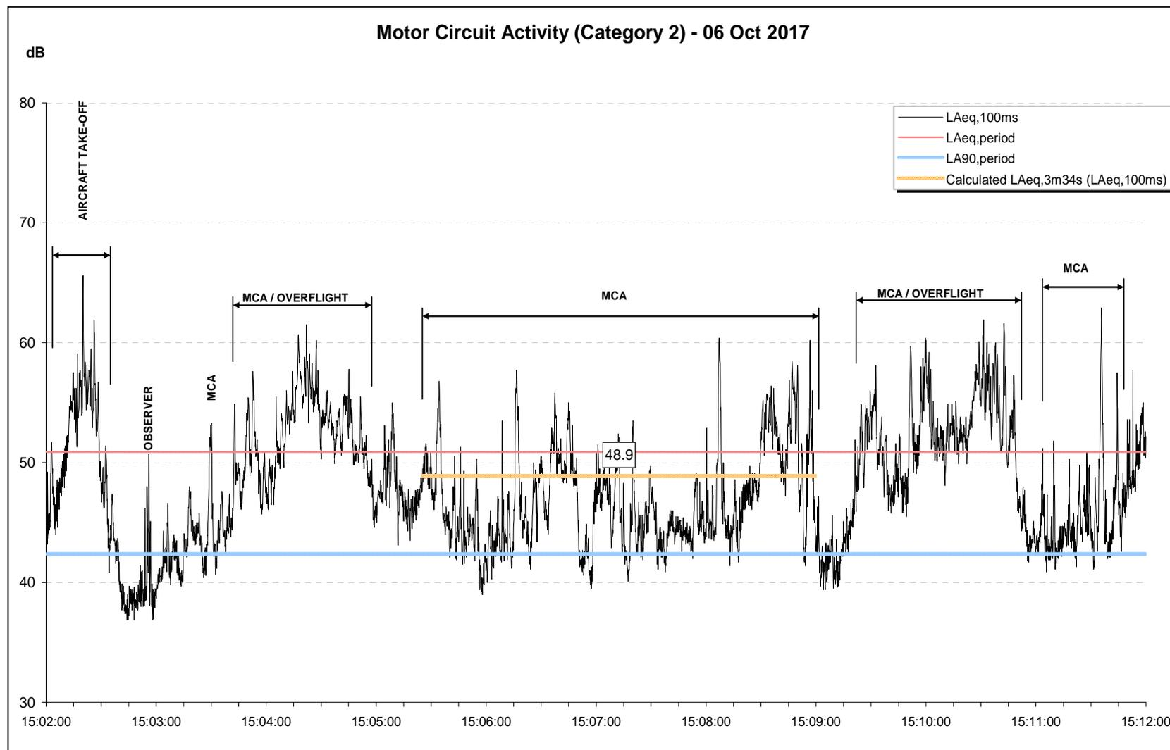
Figure 25 – Time history of motor circuit activity measured at location P5
