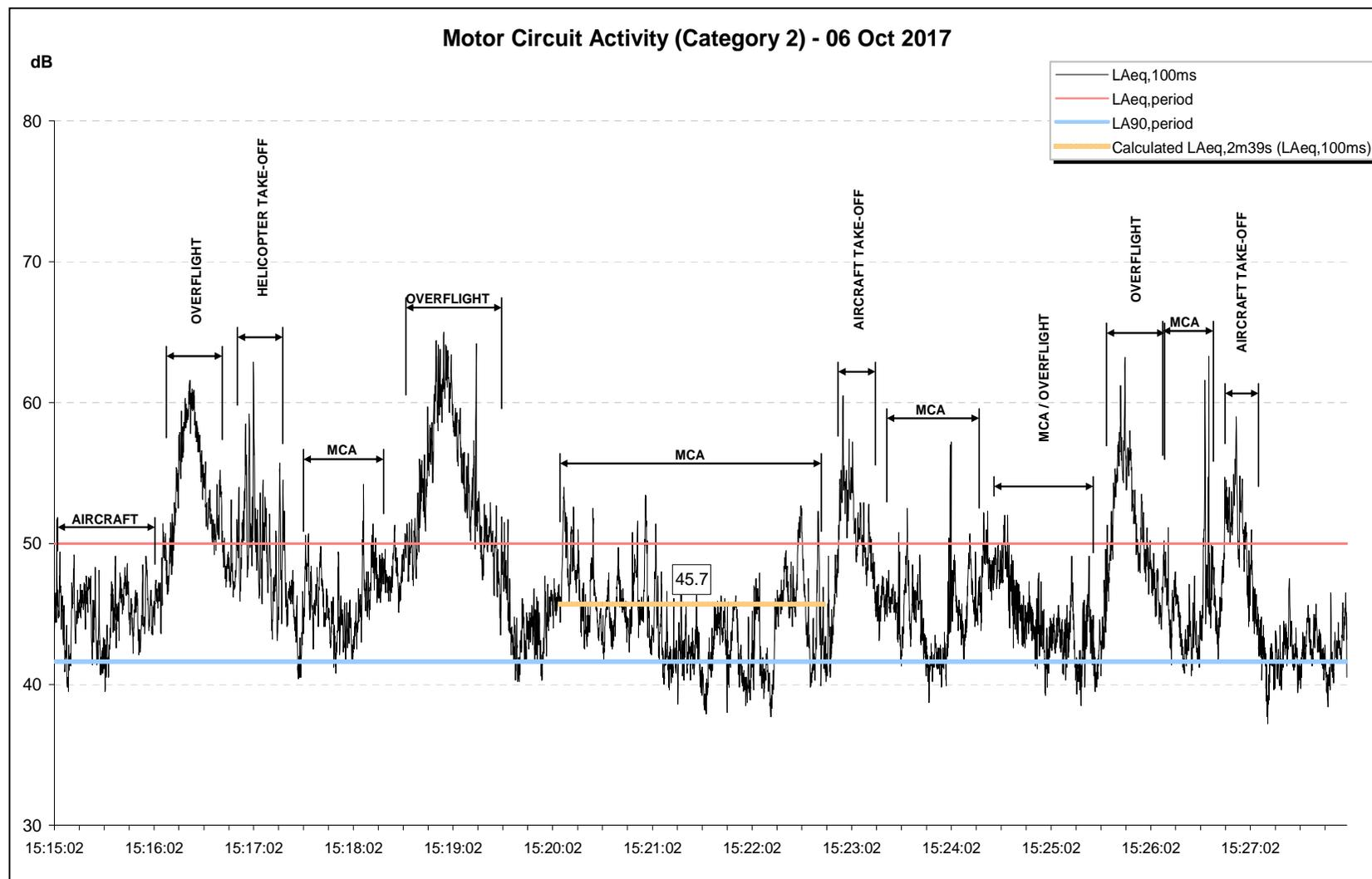
Figure 26 – Time history of motor circuit activity measured at location P6
