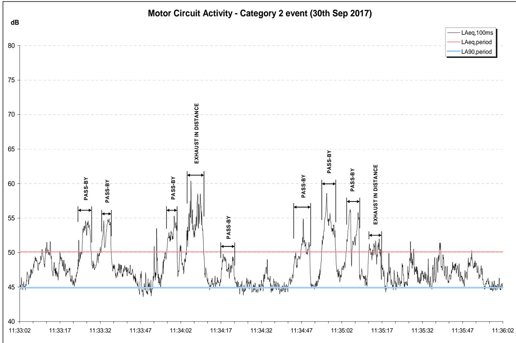
Figure 16 – Time history of motor circuit activity at meter location P3
