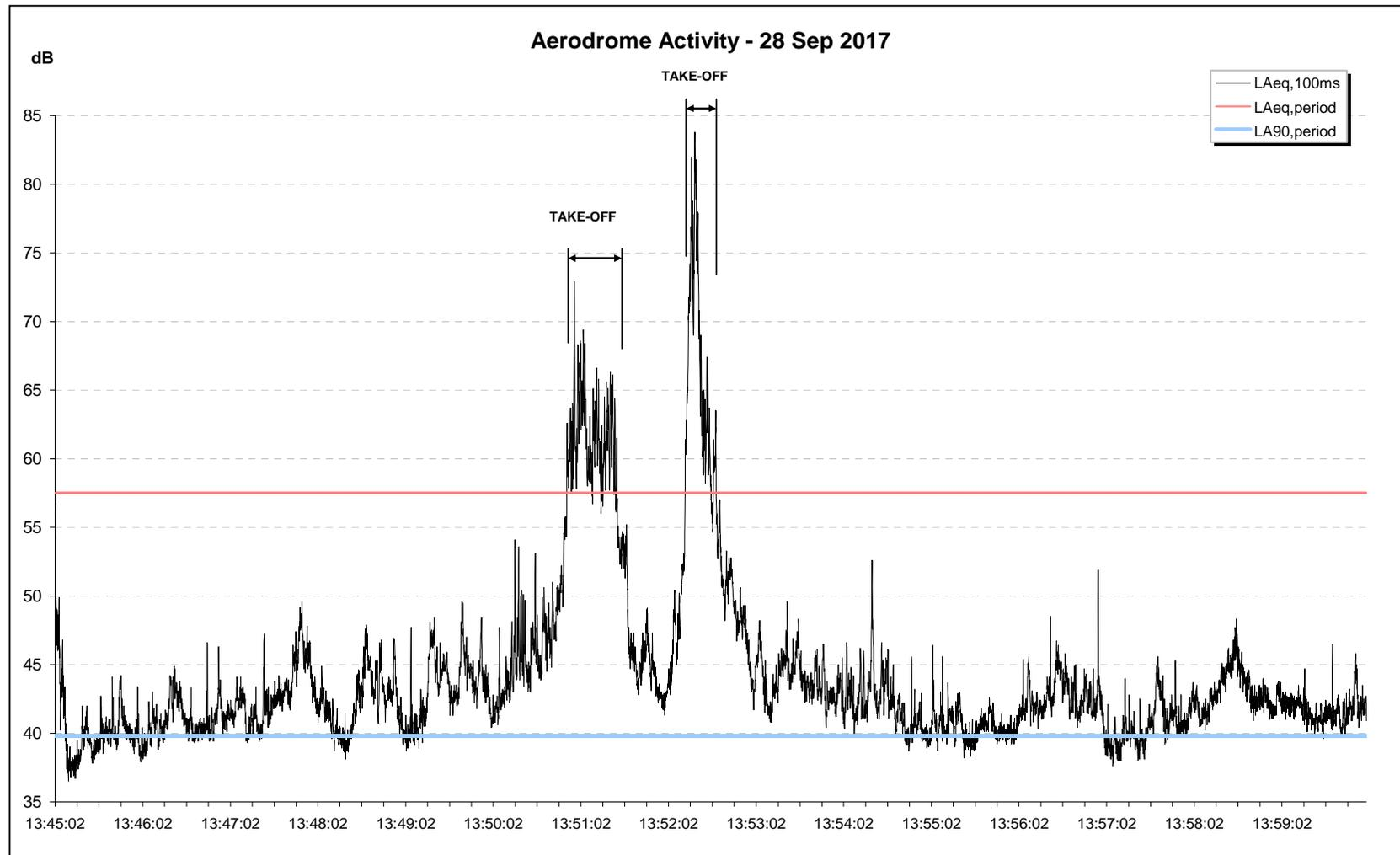
Figure 32 - Aerodrome activity measured from location F1 (28<sup>th</sup> September)
