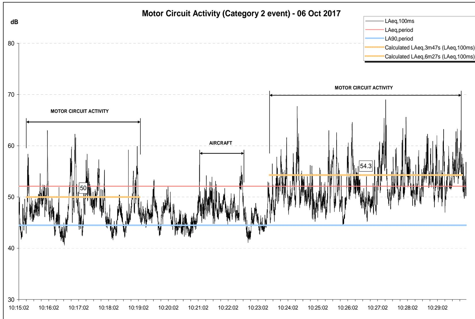
Figure 19 – Time history of motor circuit activity at location F1 (10:15 – 10:30)
