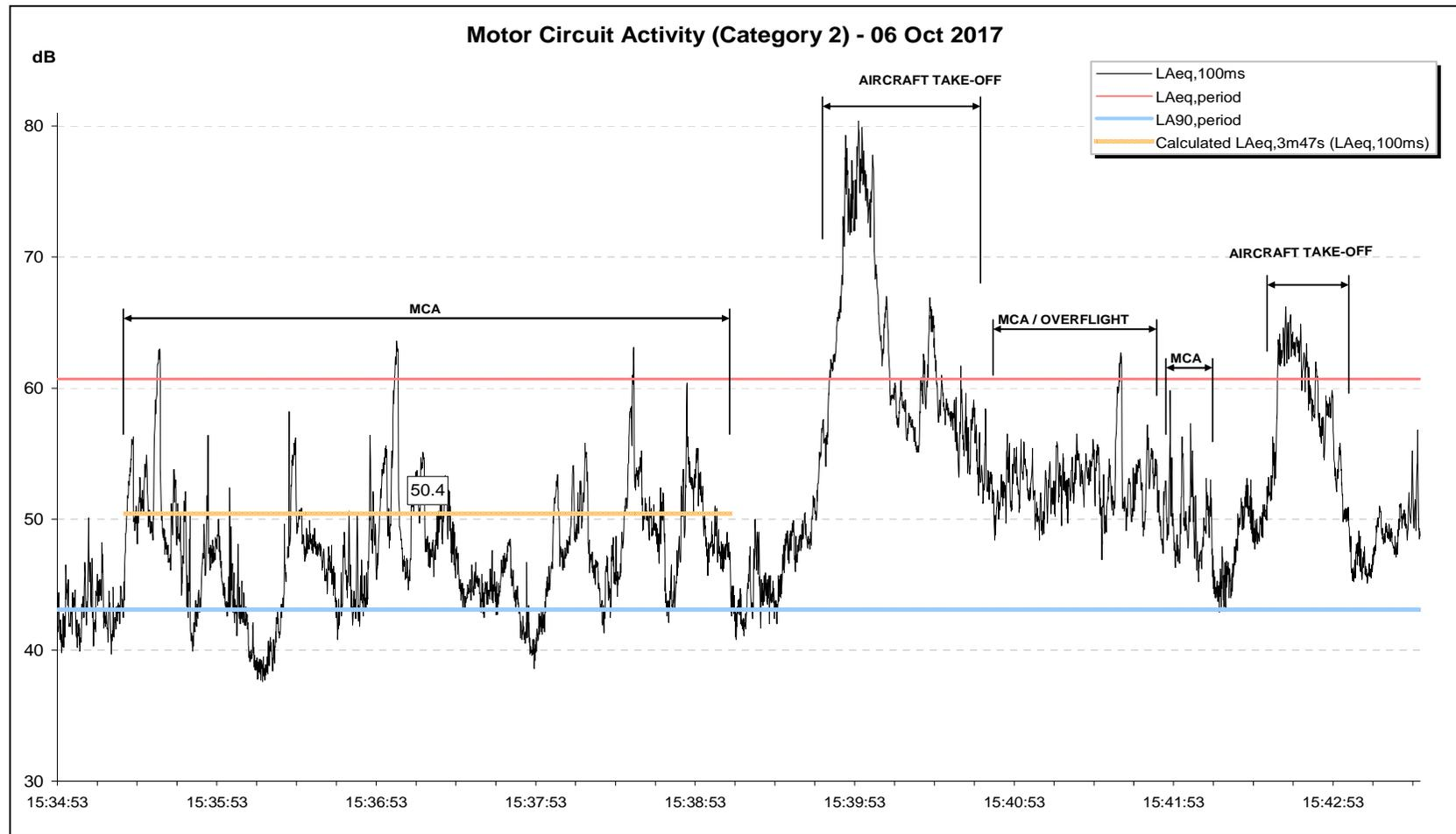
Figure 27 – Time history of motor circuit activity (MCA) measured at location P7
