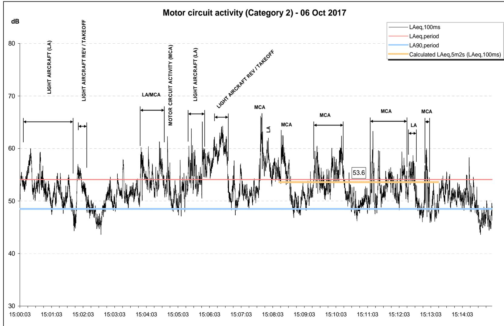
Figure 22 – Time history of motor circuit activity at location F2 (15:00 – 15:15)
