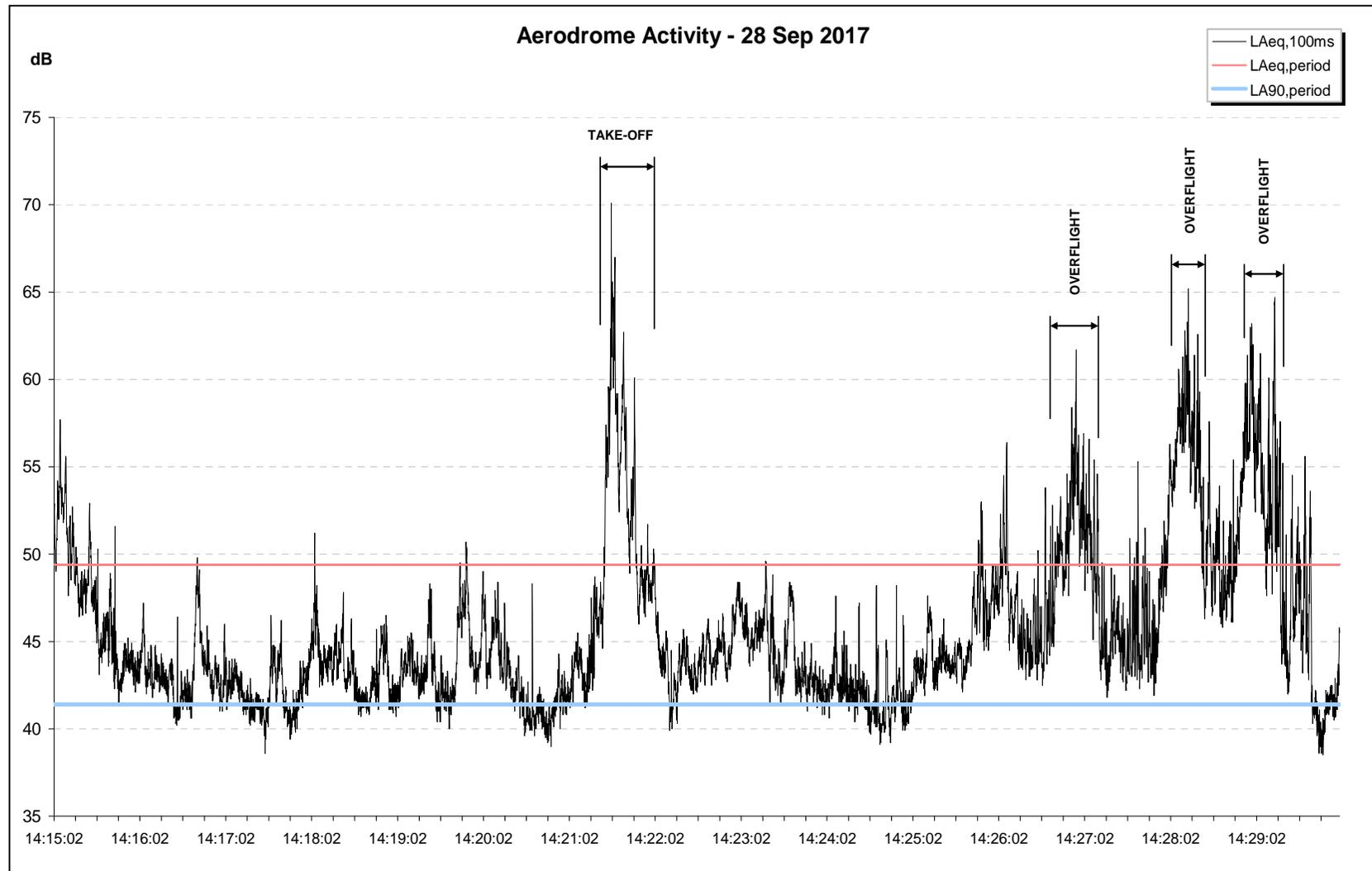
Figure 30 – Aerodrome activity measured from location F1 (28<sup>th</sup> September)
