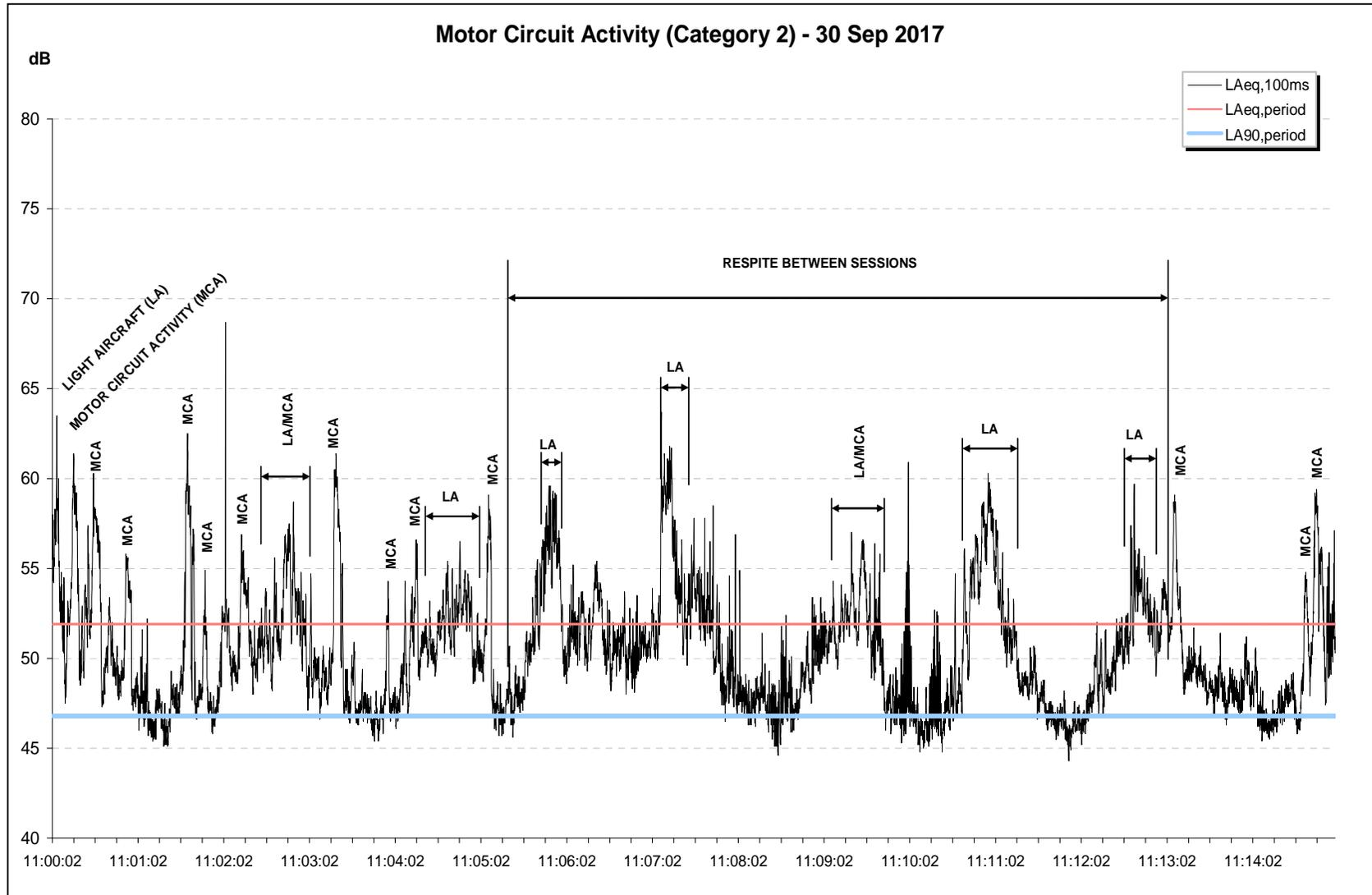
Figure 14 - Time history of motor circuit activity at meter location P1
