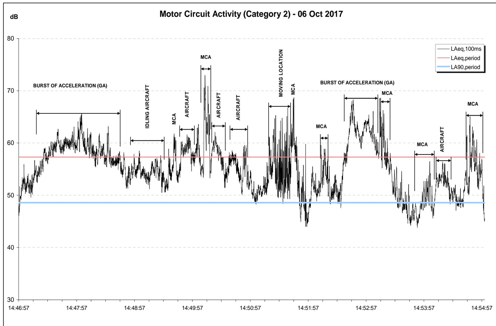
Figure 24 – Time history of motor circuit activity measured at location P4
