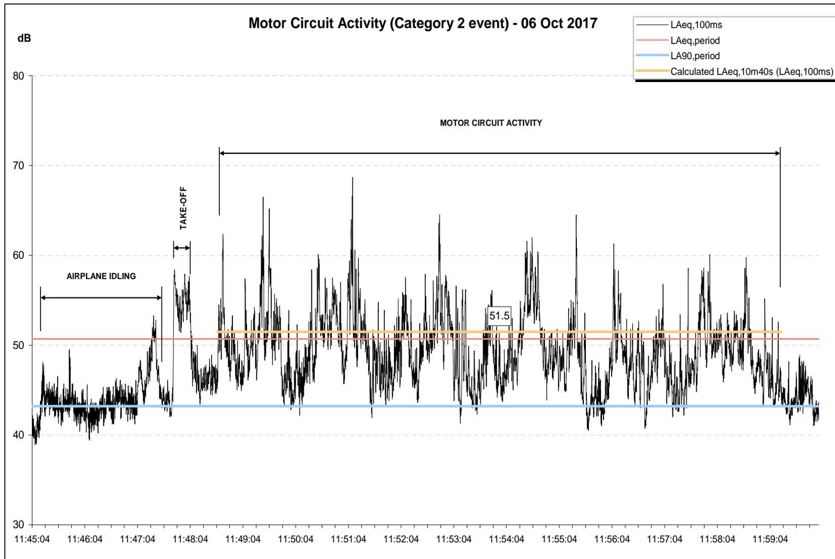
Figure 20 – Time history of motor circuit activity at location F1 (10:45 – 12:00)
