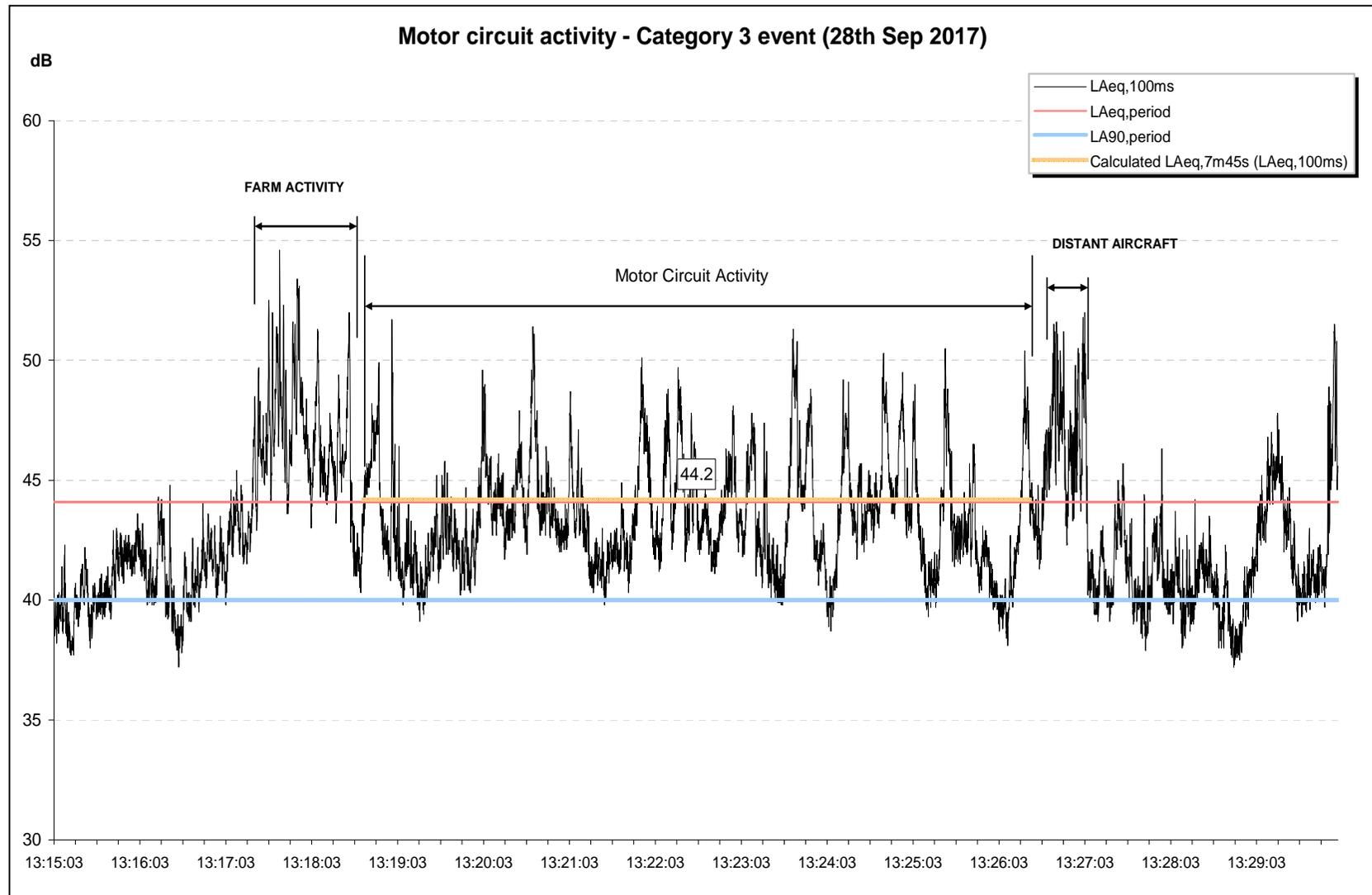
Figure 12 – Time history of motor circuit activity at meter location F1
