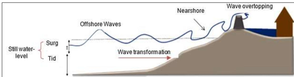
Wave overtopping is one of the principal mechanisms of flooding for the coastal frontage. The effect of wave overtopping has been included in the Flood Zone 3b delineation
