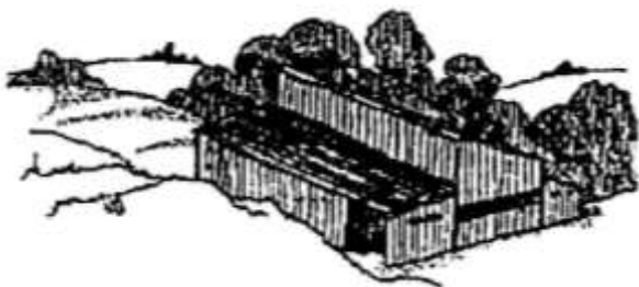
When seen against a background of trees, grey walls and darker grey roofs can help the building merge more effectively into the landscape.
