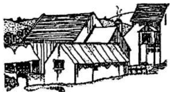
Varying roof shapes and informal irregular grouping can add visual interest and reduce regimentation and geometric shapes which are alien to undulating countryside scenery
