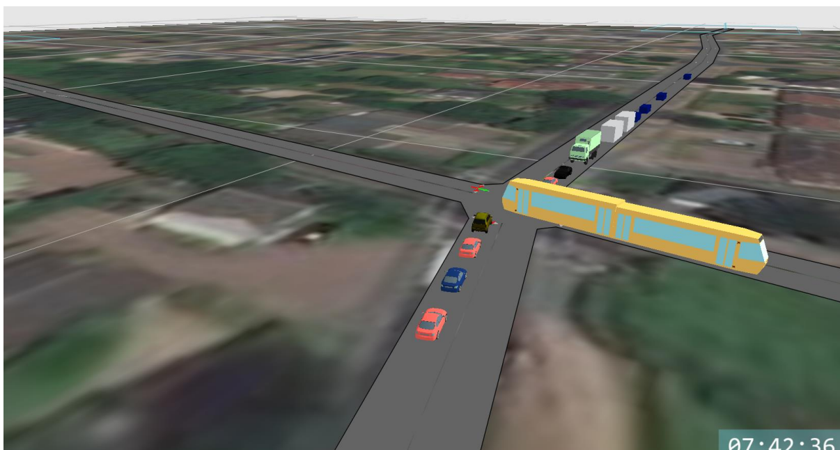
Figure 5-2: Paramics Discovery Model network snapshot with road traffic stopped as train crosses level crossing
