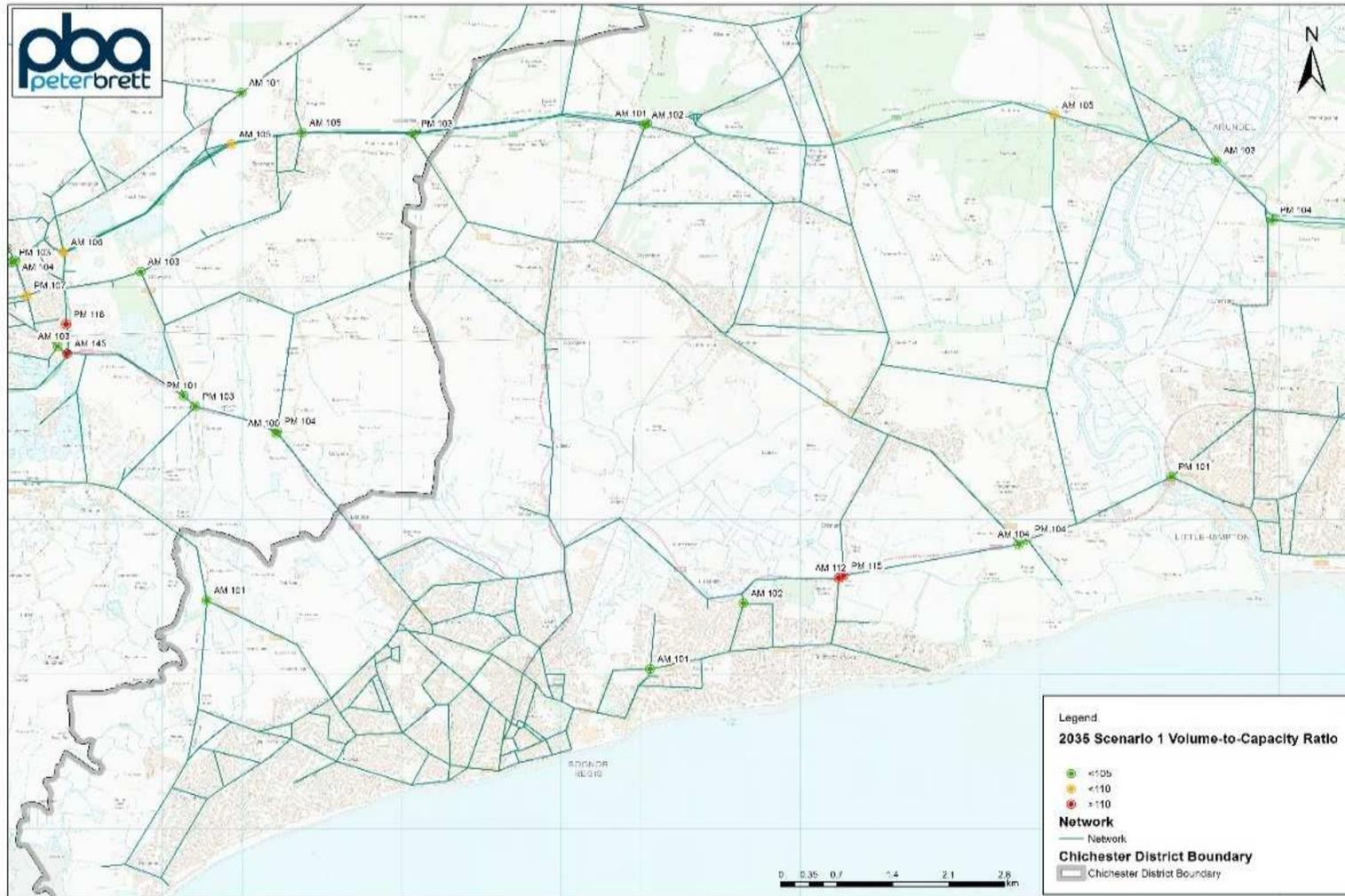
Figure 7.24: Arun Area - Volume to capacity ratios -Junction Capacity Analysis – 2035 Mitigated Scenario 1
