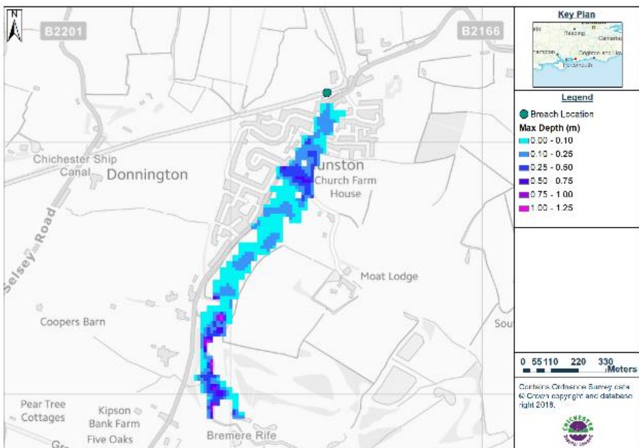
Figure 7-12: Breach modelling of the Chichester Ship Canal
