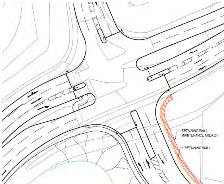
Figure 2: Initial traffic signal concept design of Cathedral Way Junction. Not to Scale.
