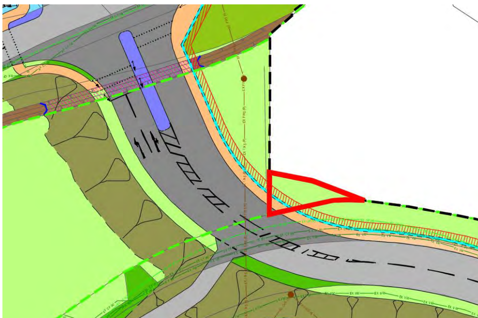
Figure 34: Overlay of Terminus Road realignment on existing Southern Water foul sewer (shown in brown) and parcel on unknown land ownership (shown with red outline)
