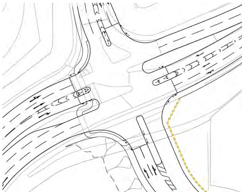
Figure 3: Proposed traffic signal concept design of Cathedral Way Junction. Not to Scale.
