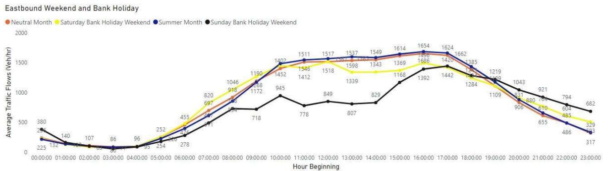
Figure 8.7: A27 Eastbound Comparison of Bank Holiday (Weekend days) flows v Weekend flows
